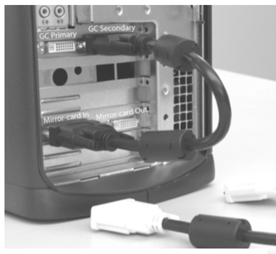
Figure 8. Short DVI cable installed.
