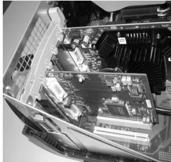
Figure 7. Mirror-flip PCI card installed.
